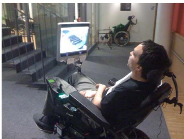
To cause the wheelchair to move, the user only needs to look at the corresponding direction zone on the screen. Additional sensors can be installed on the wheelchair in order to detect obstacles and prevent collisions with walls and other people.
