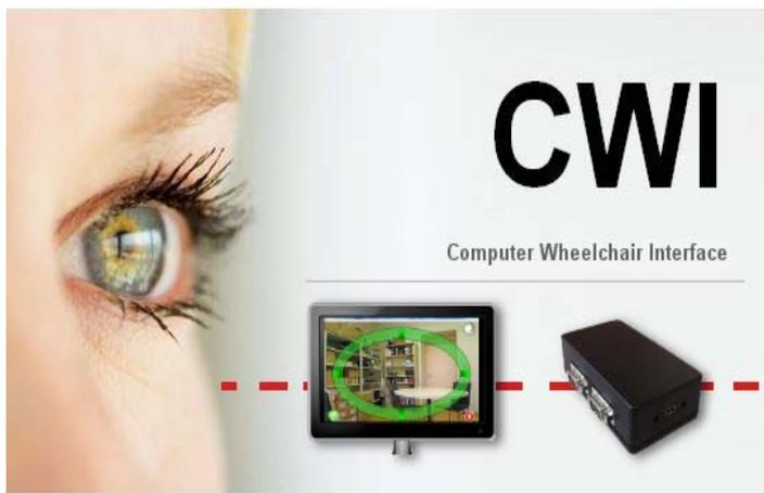
**CWI (Computer Wheelchair Interface)** is an innovative mobility interface that enables autonomous eye-controlled wheelchair navigation. By using eye tracking techniques, CWI detects the direction the user looks at and moves the electric wheelchair accordingly.
